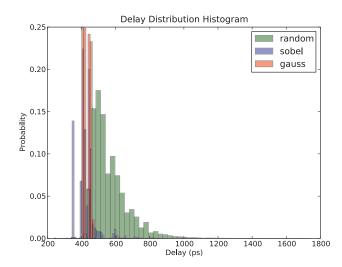
Fig. 2. Delay distribution of INT\_ADD under three different input workload sets.
